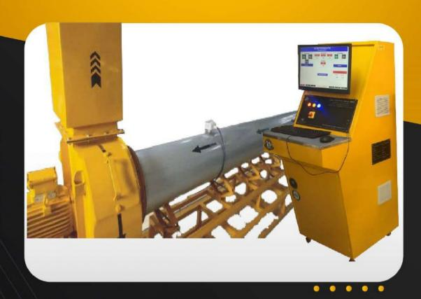
**HVAC Air Filter Test Rig**
