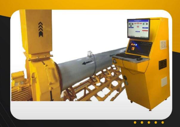
**HVAC Air Filter Test Rig**
