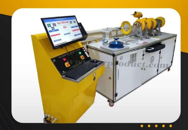
Air Filter Flat Sheet Media Test Equipment
